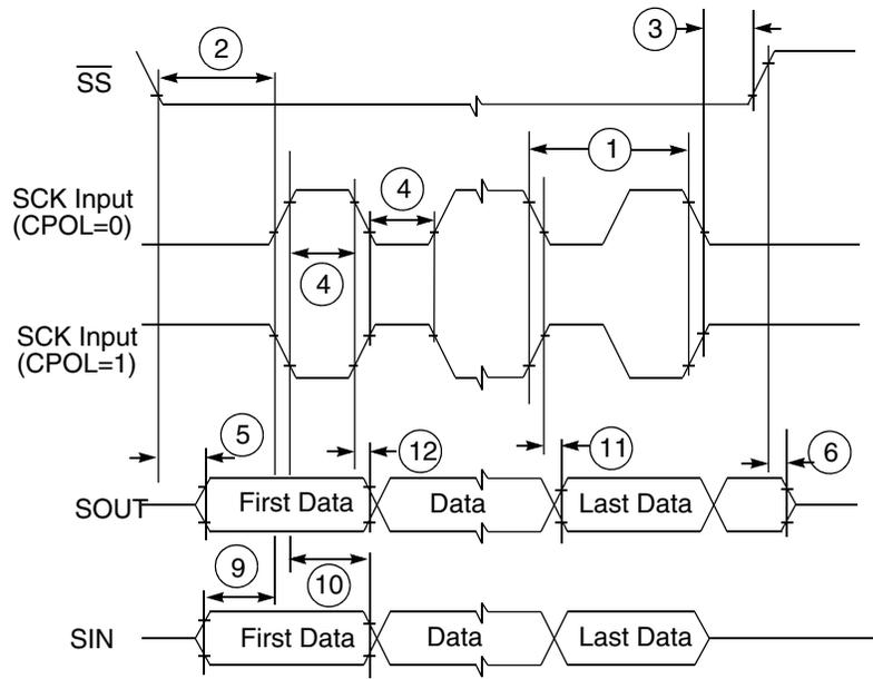
**Figure 12. SPI classic SPI timing — slave, CPHA = 0**
