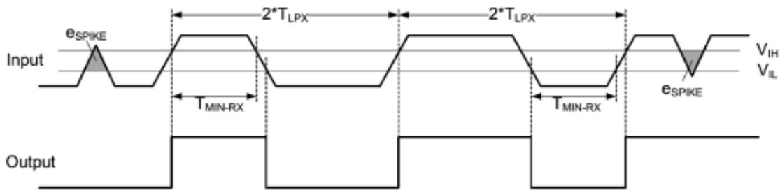
**Figure 26. Input Glitch Rejection of Low-Power Receivers**
