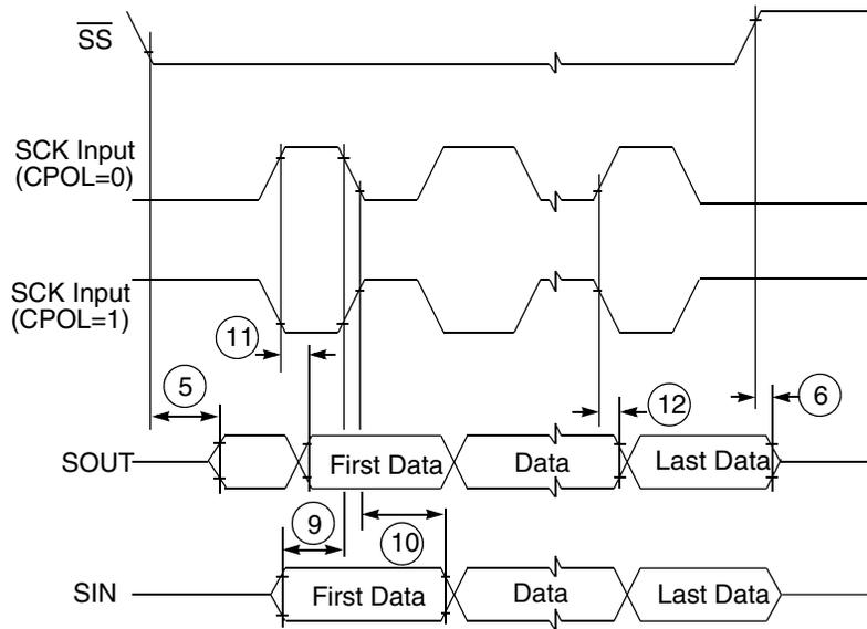
**Figure 13. SPI classic SPI timing — slave, CPHA = 1**
