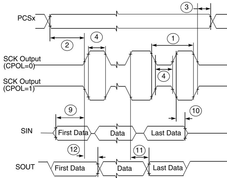
**Figure 14. SPI modified transfer format timing — master, CPHA = 0**
