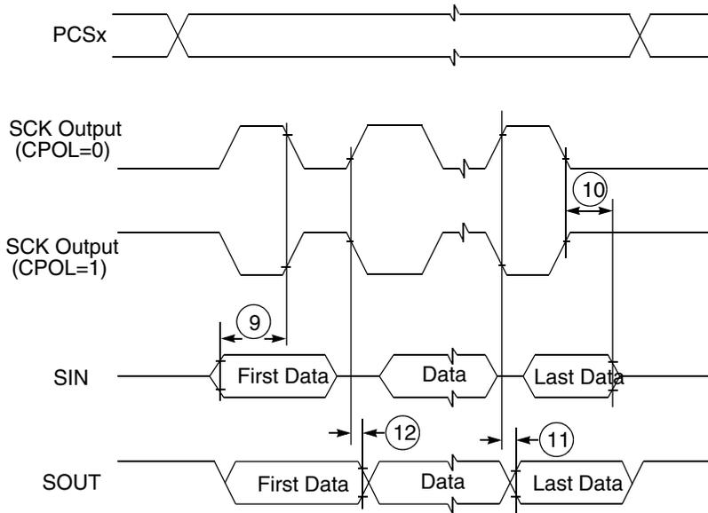
**Figure 11. SPI classic SPI timing — master, CPHA = 1**
