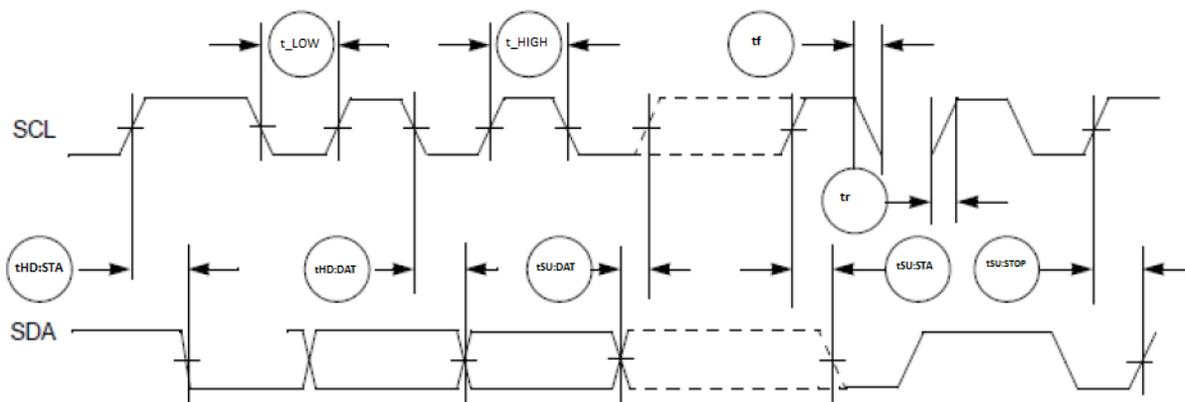
Figure 17. I<sup>2</sup>C input/output timing
