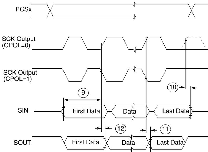
**Figure 15. SPI modified transfer format timing — master, CPHA = 1**
