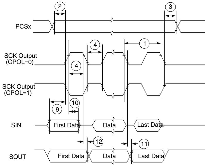
**Figure 10. SPI classic SPI timing — master, CPHA = 0**
