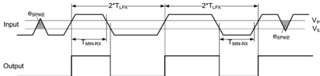
**Figure 26. Input Glitch Rejection of Low-Power Receivers**
