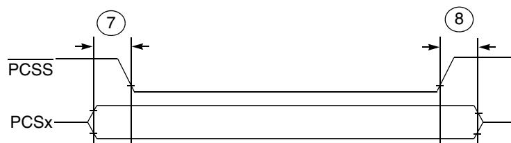
**Figure 16. SPI PCS strobe (PCSS) timing**
