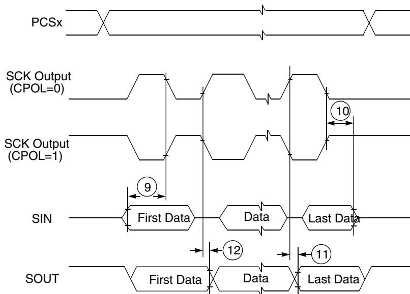
**Figure 11. SPI classic SPI timing — master, CPHA = 1**
