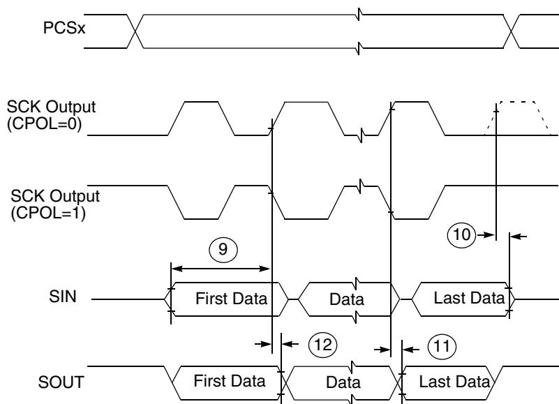
**Figure 15. SPI modified transfer format timing — master, CPHA = 1**
