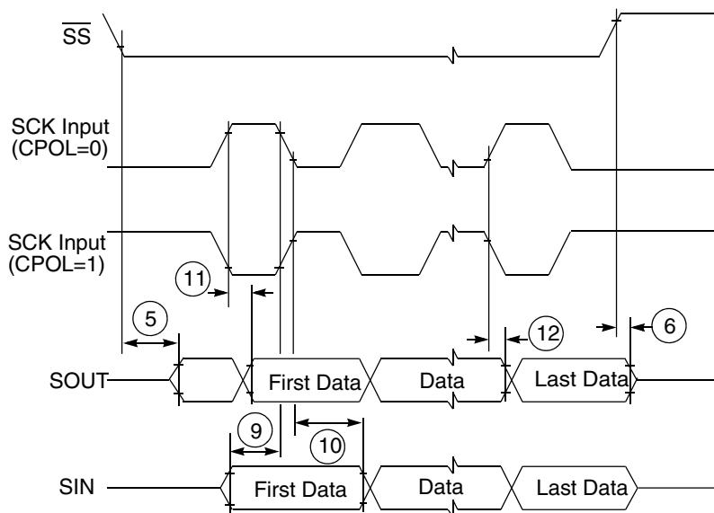
**Figure 13. SPI classic SPI timing — slave, CPHA = 1**
