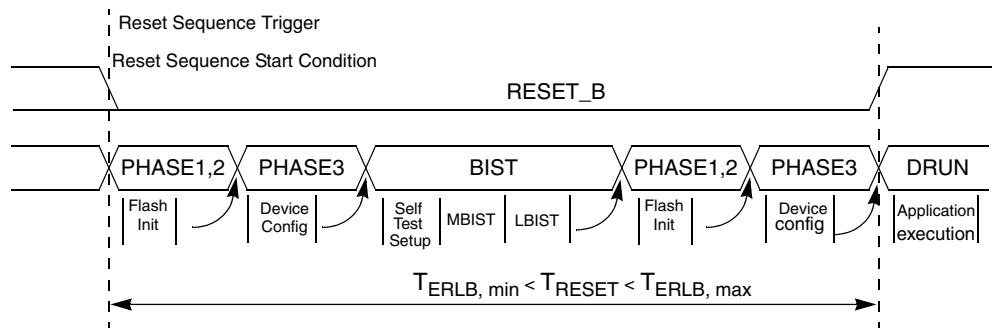
**Figure 30. External reset sequence long, BIST enabled**
