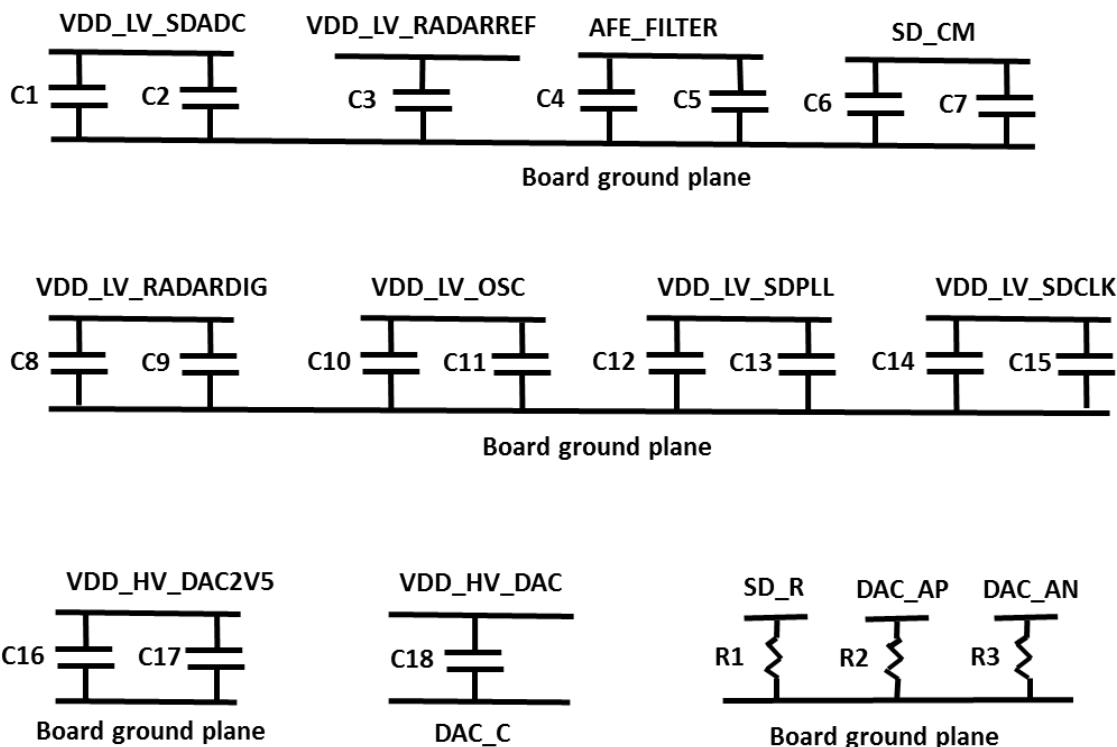
**Figure 4. Radar AFE External Components Configuration****Table 10. Radar AFE External Components**
