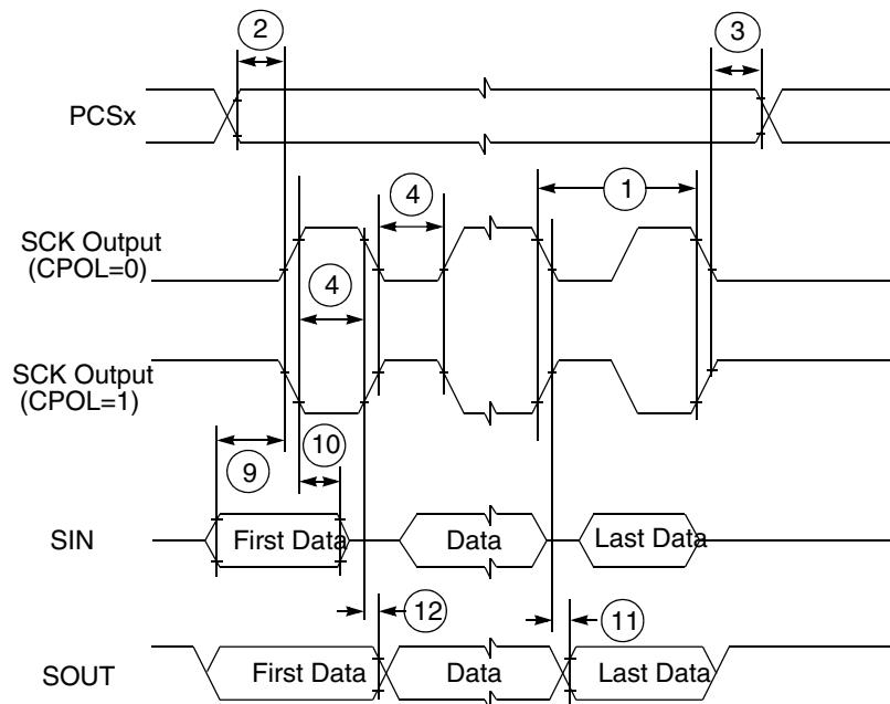
**Figure 10. SPI classic SPI timing — master, CPHA = 0**
