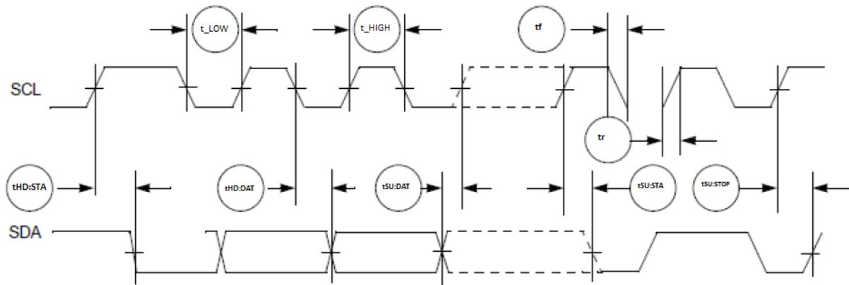
Figure 17. I<sup>2</sup>C input/output timing
