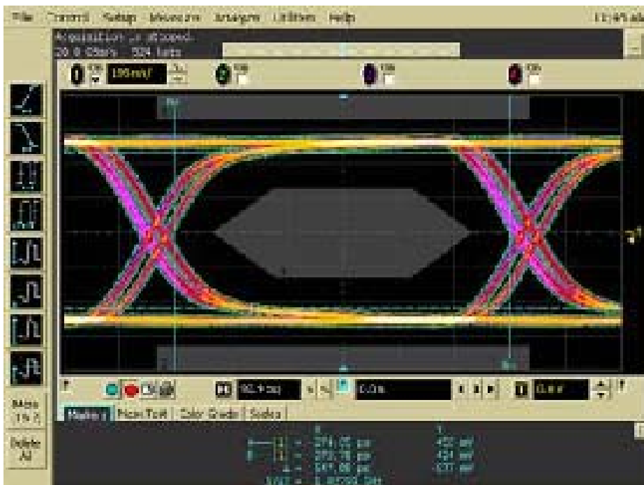
Figure 4: 8bit deep color DVI/HDMI TX eye tested with 10 meter. 24 AWG HDMI cable. Setting: Optimized equalization, 0dB output pre-emphasis and de-emphasis, and Swing 500mV.
