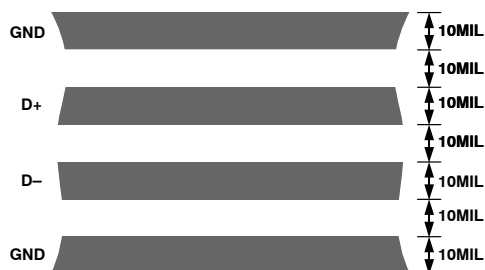
Figure 19. Arrangement of Signal Tracks
