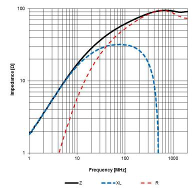
Test Equipment: E4991A or equivalent
