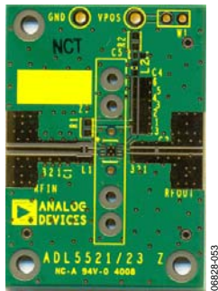
Figure 55. Evaluation Board Layout (Top View)
