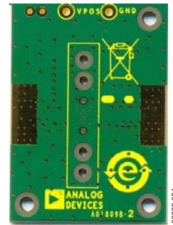
Figure 56. Evaluation Board Layout (Bottom View)
