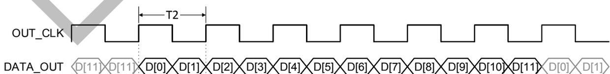
Figure 19: 12-bit pixel data on an LVDS channel
