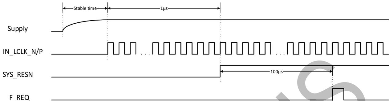
Figure 7: Start-up sequence for 600Mbps @ 10-bit
