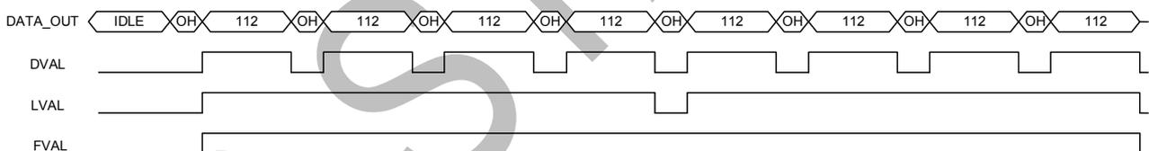
Figure 33: DVAL, LVAL and FVAL timing in 8 output mode
