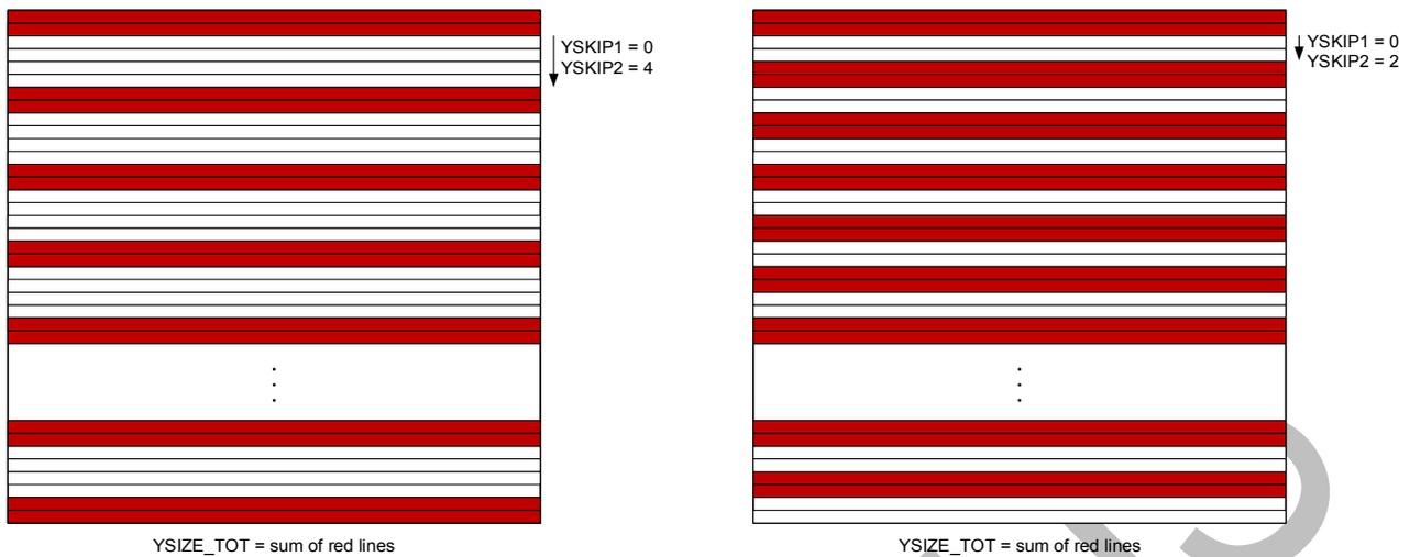
Figure 44: Subsampling examples in advanced mode (skip 4x and skip 2x)
