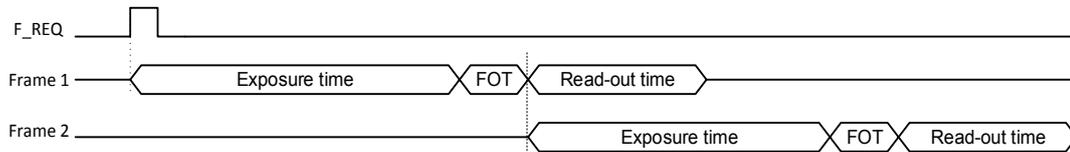
Figure 14: request for 2 frames in internal exposure mode
