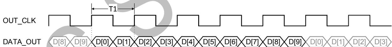
Figure 18: 10-bit pixel data on an LVDS channel
