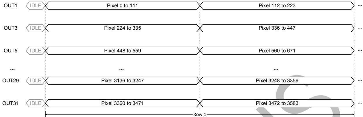
Figure 28: Pixel remapping for 16 output channels
