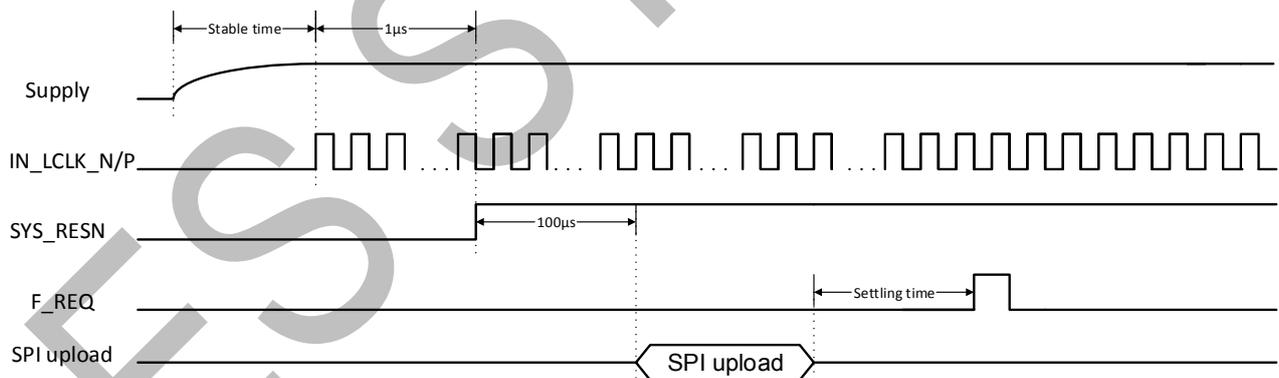
Figure 8: Start-up sequence for 12 bit mode
