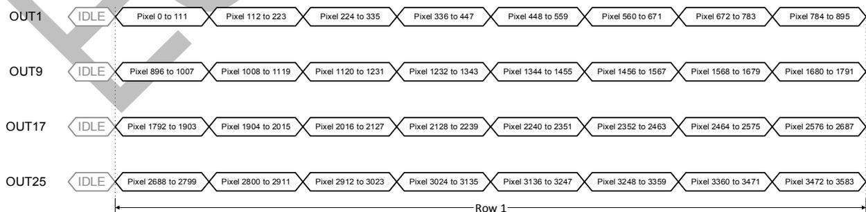
Figure 30: Pixel remapping for 4 output channels
