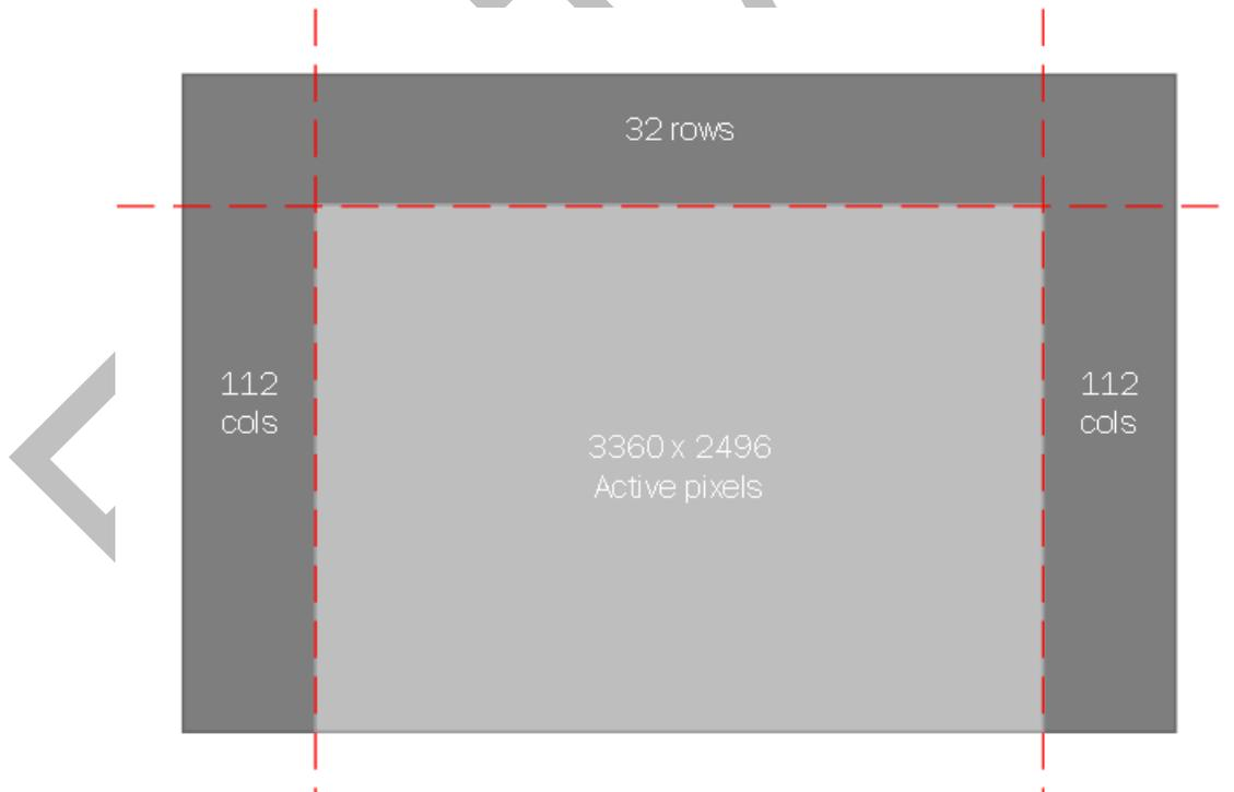
**Figure 4 Logical organization of the pixel array**
