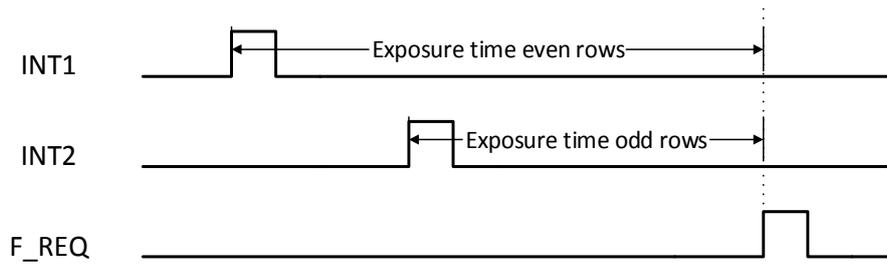
Figure 36: Interleaved read-out in external exposure mode
