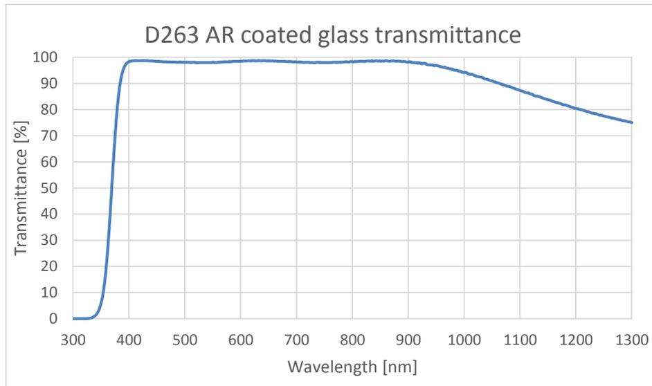
Figure 48: Transmittance curve of D263 AR-coated cover glass
