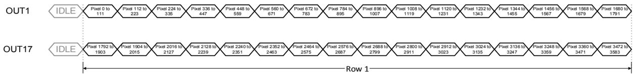
Figure 31: Pixel remapping for 2 output channels
