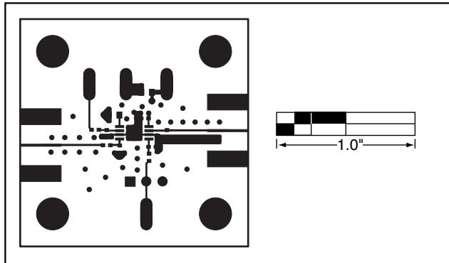
Figure 3. MAX2754 EV Kit PC Board Layout—Component Side
