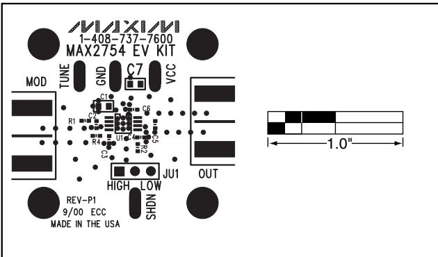
Figure 2. MAX2754 EV Kit Component Placement Guide—Top Silkscreen
