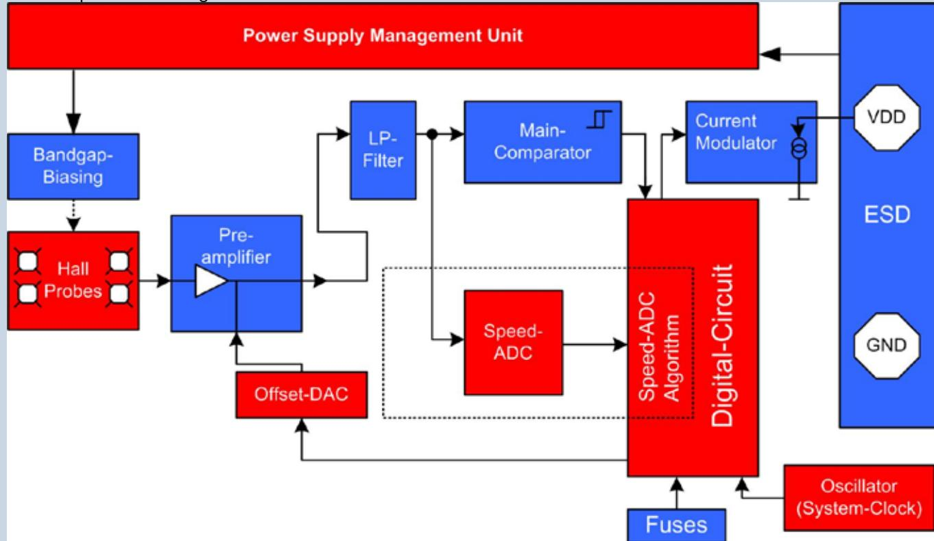
The TLE4941plusC signal path includes a pair of hall probes (2 mm spacing), a differential amplifier and a comparator feeding a switched current output stage. Additionally, the circuit has a feedback loop for offset compensation which consists of a signal-Speed ADC, a digital signal processor (DSP) and an offset D/A converter.
