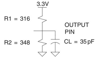
Note: Similar devices are tested with slightly different loads. These load differences may affect output signals' delay and slew rate. Atmel devices are tested with sufficient margins to meet compatible devices.
