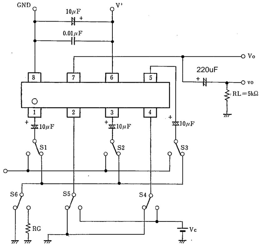
This IC requires  $1M\Omega$  resistance between INPUT and GND pin for clamp type input since the minute current causes an unstable pin voltage.
