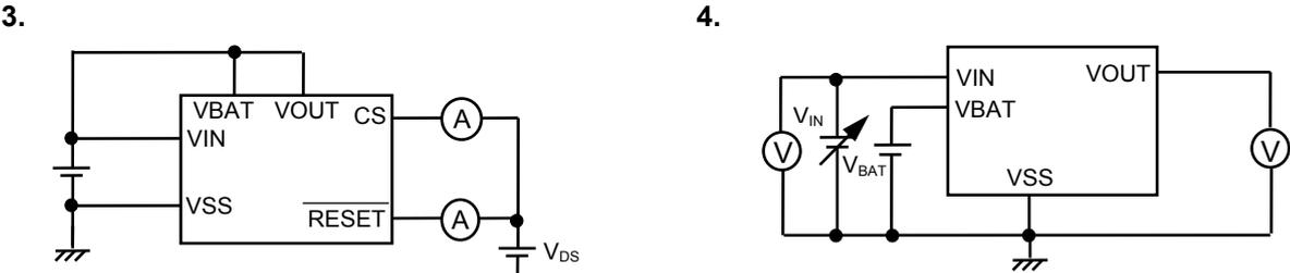
Measure the value after applying 6 V to VIN.
