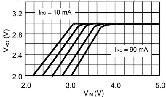
**1.2 Input Voltage ( $V_{IN}$ ) vs. Output Voltage ( $V_{OUT}$ ) Characteristics (REG2) ( $V_{OUT} = 3.0\text{ V}$ )**
