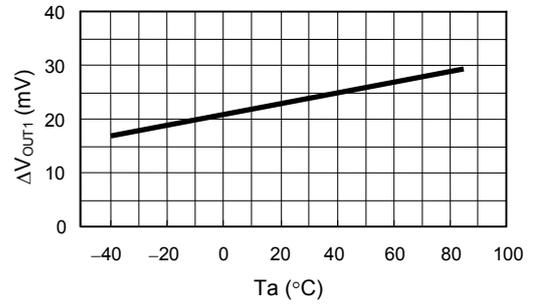
**1.18 Load Stability ( $\Delta V_{CH1}$ ) Temperature Characteristics**
