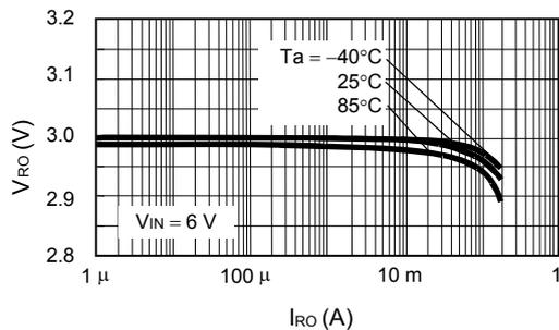
**1.8 Output Current ( $I_{OUT}$ ) vs. Output Voltage ( $V_{OUT}$ ) Characteristics**
