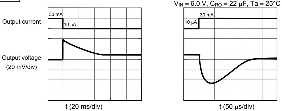
**Figure 23 Ringing Waveform due to Load Variation (VRO Pin)**
