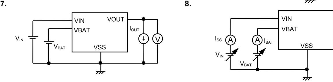
Leave open and measure the value after applying 6 V to VIN.
