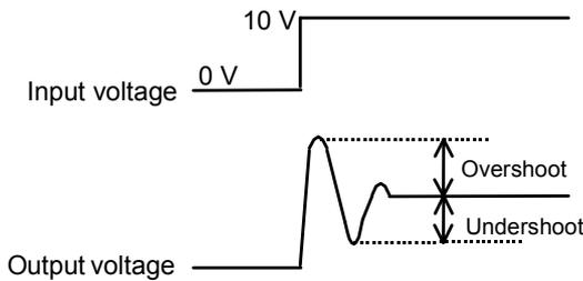
Figure 10 Power Supply Application: 0 V→10 V Square Wave
