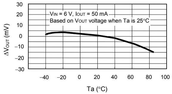
**1.12 Output Voltage ( $V_{CH}$ ) Temperature Characteristics**
