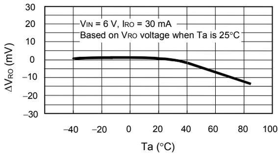
**1.11 Output Voltage ( $V_{OUT}$ ) Temperature Characteristics**
