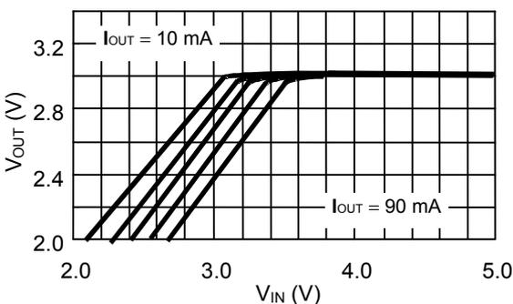
1.3 Input Voltage ( $V_{IN}$ ) vs. Output Voltage ( $V_{OUT}$ ) Characteristics (REG3) ( $V_{CH} = 3.3\text{ V}$ )
