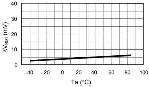
**1.17 Load Stability ( $\Delta V_{OUT1}$ ) Temperature Characteristics**
