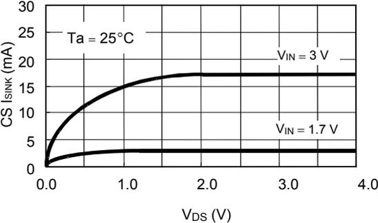
(3) Output current ( $I_{SINK}$ ) temperature characteristics
