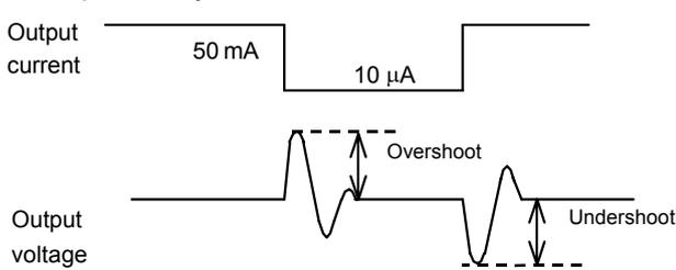
**Figure 20 Output Voltage Variation due to Output Current**
