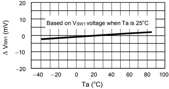
**3.2 CS Output Inhibit Voltage ( $V_{SW2}$ ) Temperature Characteristics**
