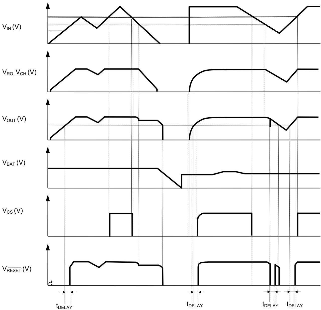
**Remark** CS and  $\overline{RESET}$  are pulled up to  $V_{OUT}$ . The Y-axis is an arbitrary scale.
