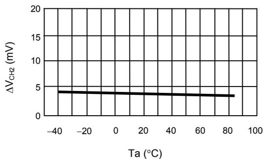
**1.16 Load Stability ( $\Delta V_{RO1}$ ) Temperature Characteristics**
