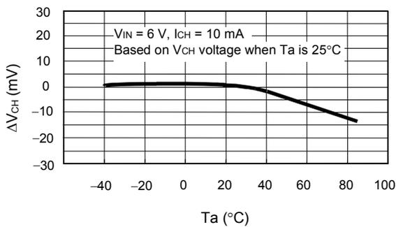
**1.13 Input Stability ( $\Delta V_{RO2}$ ) Temperature Characteristics**
