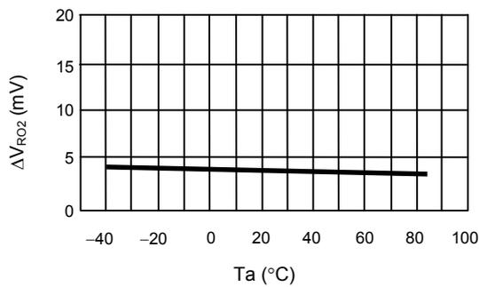
**1.14 Input Stability ( $\Delta V_{OUT2}$ ) Temperature Characteristics**
