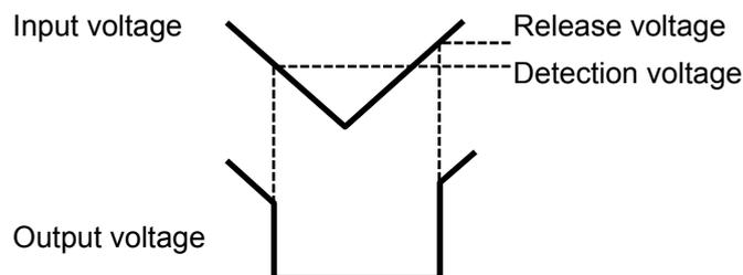
Figure 6 Definition of Detection and Release Voltages
