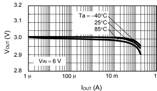
**1.9 Output Current ( $I_{OUT}$ ) vs. Output Voltage ( $V_{CH}$ ) Characteristics**
