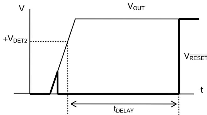
**Figure 7 Definition of  $\overline{\text{RESET}}$  Release Delay Time ( $t_{\text{DELAY}}$ )**
