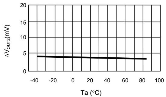
**1.15 Input Stability ( $\Delta V_{CH2}$ ) Temperature Characteristics**
