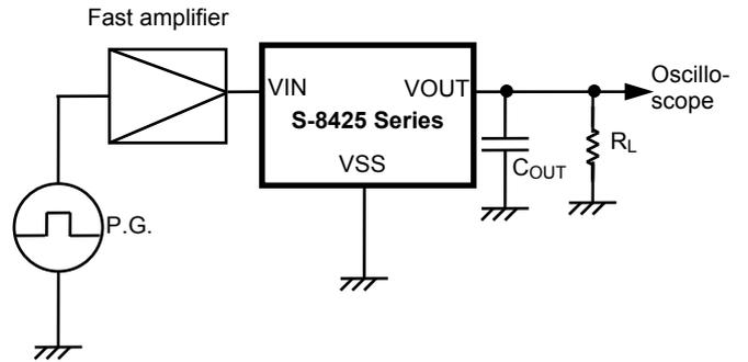
**Figure 16 Test Circuit**
