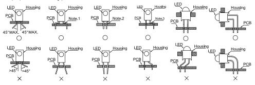
"  $\bigcirc$  " Correct mounting method " imes " Incorrect mounting method
