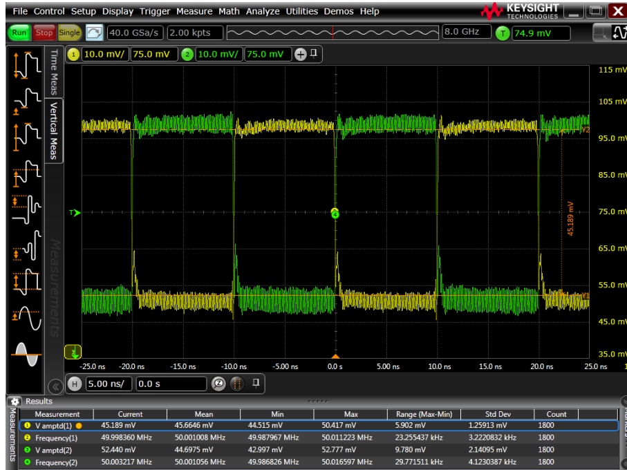
Figure 5-3. LVDS 2.5 V, 50 MHz Clock Measured with DC Coupling, 50-Ω Scope Termination
