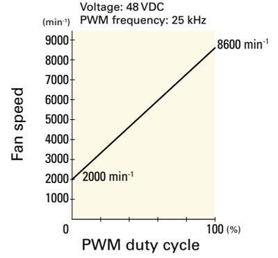
**9SG5748P5H01** With pulse sensor with PWM control function
