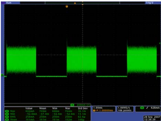
FIGURE 11. IL AT 50% PWM DIMMING
