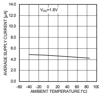
Fig.16 I<sub>DD</sub>– Ambient temperature
