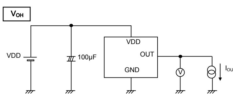
Fig.3 V<sub>OH</sub> measurement circuit
