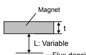
Fig.71 Magnet Dimensions and Flux Density Measuring Point
