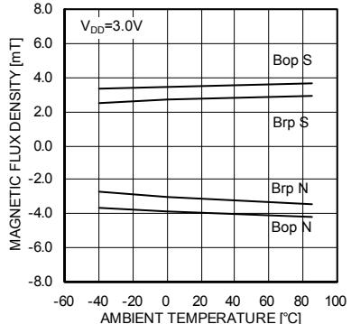
Fig.24 Bop,Brp–Ambient temperature
