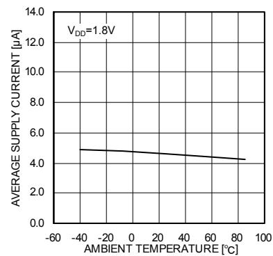
Fig.40 I<sub>DD</sub>– Ambient temperature
