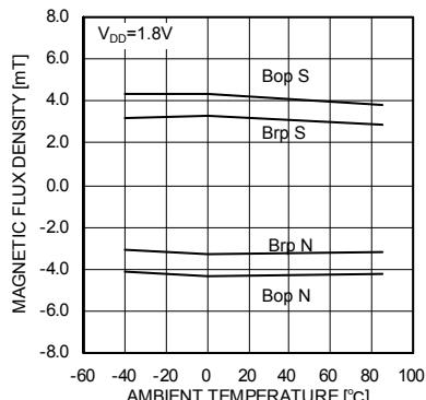
Fig.12 Bop,Brp– Ambient temperature
