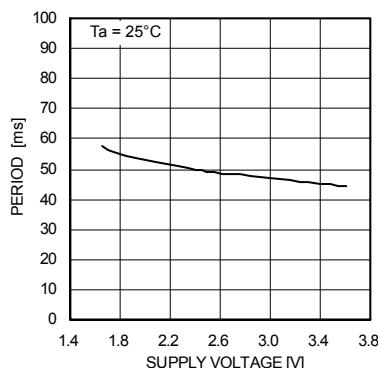
Fig.39 T<sub>P</sub>– Supply voltage
