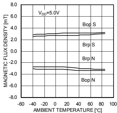
Fig.54 Bop,Brp–Ambient temperature
