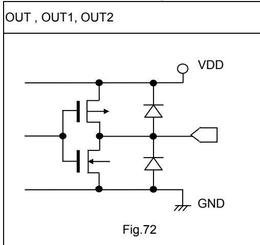
Because they are configured for CMOS (inverter) output, the output pins require no external resistance and allow direct connection to the PC. This, in turn, enables reduction of the current that would otherwise flow to the external resistor during magnetic field detection, and supports overall low current (micropower) operation.
