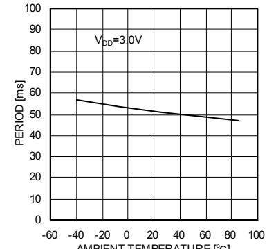
Fig.26  $T_P$  – Ambient temperature
