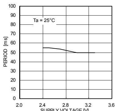
Fig.27  $T_P$  – Supply voltage
