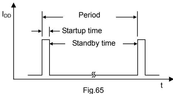
The bipolar detection Hall IC adopts an intermittent operation method to save energy. At startup, the Hall elements, amp, comparator and other detection circuits power ON and magnetic detection begins. During standby, the detection circuits power OFF, thereby reducing current consumption. The detection results are held while standby is active, and then output.
