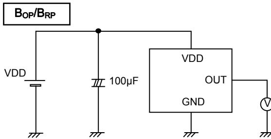
Bop and Brp are measured with applying the magnetic field from the outside.
