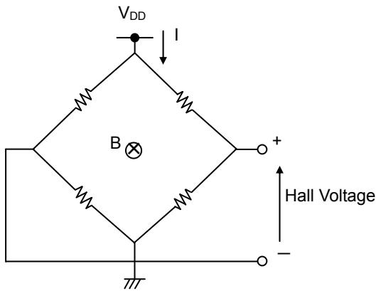
The Hall elements form an equivalent Wheatstone (resistor) bridge circuit. Offset voltage may be generated by a differential in this bridge resistance, or can arise from changes in resistance due to package or bonding stress. A dynamic offset cancellation circuit is employed to cancel this offset voltage.
