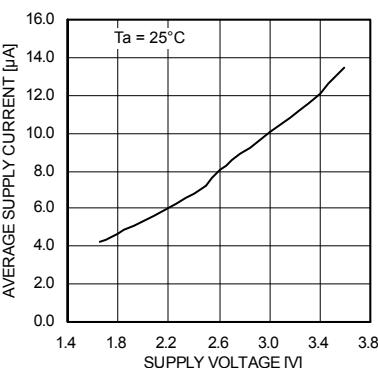
Fig.41 I<sub>DD</sub> – Supply voltage
