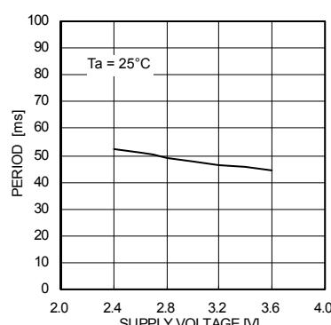
Fig.51 T<sub>P</sub> – Supply voltage
