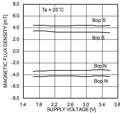
Fig.13 Bop,Brp– Supply voltage
