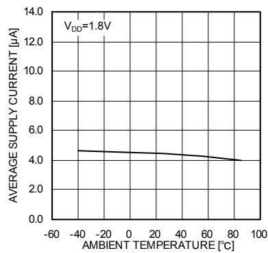
Fig.46 I<sub>DD</sub> – Ambient temperature
