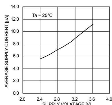
Fig.53 I<sub>DD</sub> – Supply voltage
