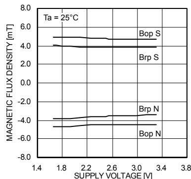
Fig.43 Bop,Brp – Supply voltage
