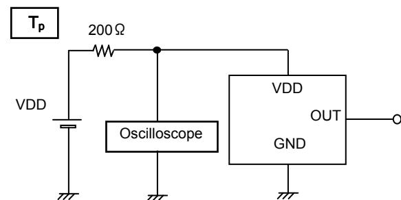
The period is monitored by Oscilloscope.
