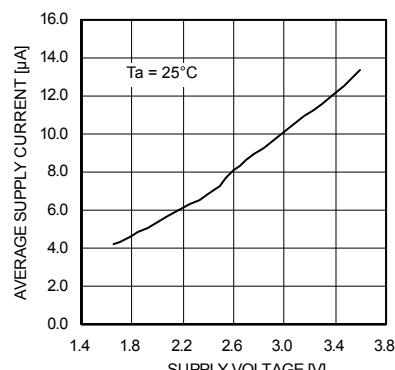
Fig.11 I<sub>DD</sub>– Supply voltage
