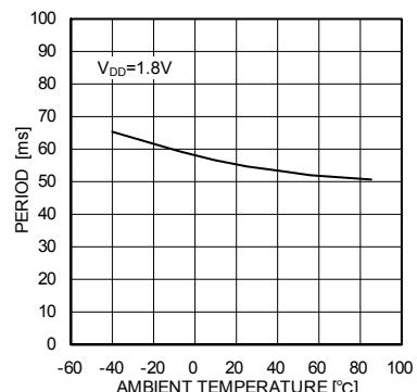
Fig.44 T<sub>P</sub> – Ambient temperature
