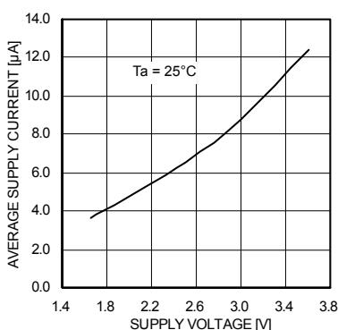
Fig.35 I<sub>DD</sub> – Supply voltage
