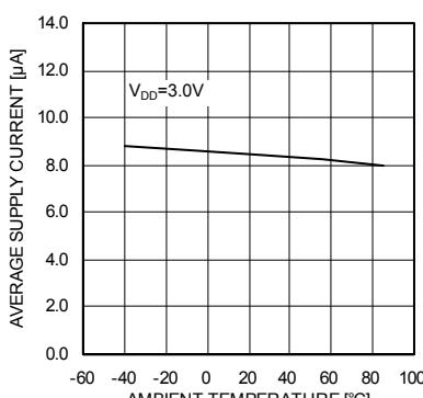
Fig.28  $I_{DD}$  – Ambient temperature
