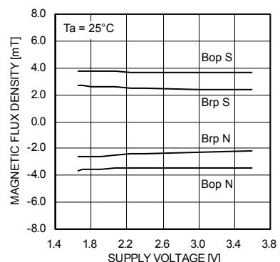
Fig.31 Bop,Brp– Supply voltage
