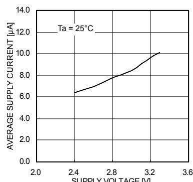
Fig.29  $I_{DD}$  – Supply voltage
