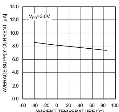
Fig.52 I<sub>DD</sub> – Ambient temperature
