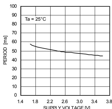
Fig.33 T<sub>P</sub>– Supply voltage
