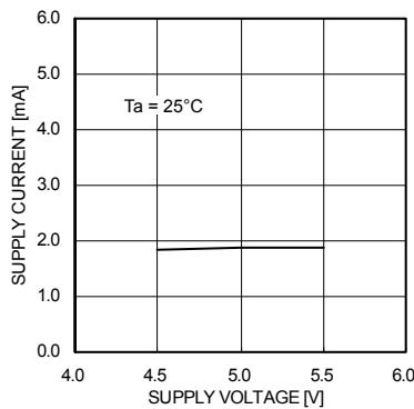
Fig.57 I<sub>DD</sub> – Supply voltage
