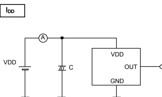
Fig.5 I<sub>DD</sub> measurement circuit
