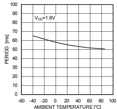
Fig.8 T<sub>P</sub>– Ambient temperature
