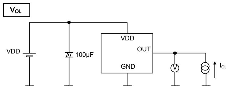
Fig.4 V<sub>OL</sub> measurement circuit
