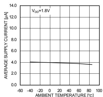
Fig.34 I<sub>DD</sub>– Ambient temperature
