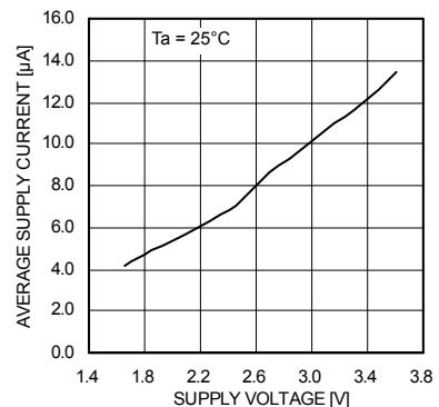
Fig.17 I<sub>DD</sub>– Supply voltage
