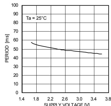
Fig.15 T<sub>P</sub>– Supply voltage
