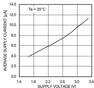
Fig.47 I<sub>DD</sub> – Supply voltage
