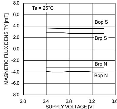
Fig.25 Bop,Brp– Supply voltage
