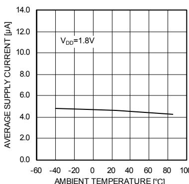
Fig.10 I<sub>DD</sub>– Ambient temperature
