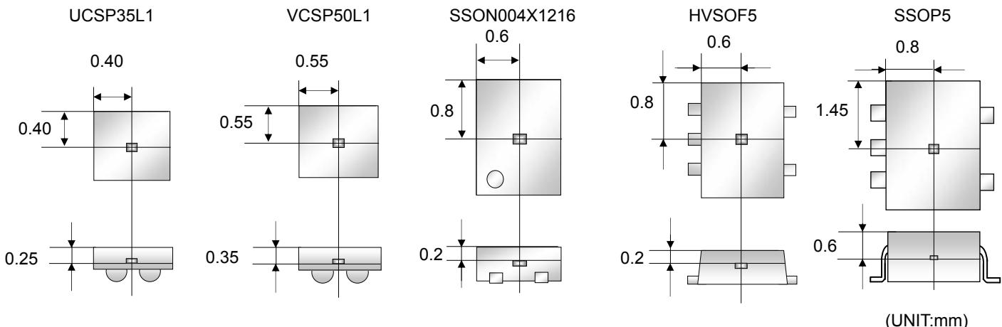
●Footprint dimensions (Optimize footprint dimensions to the board design and soldering condition)
