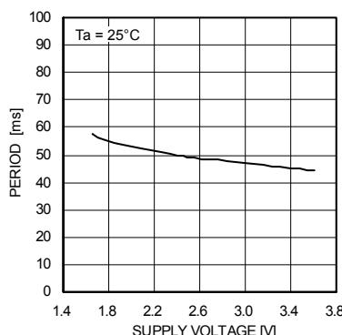
Fig.45 T<sub>P</sub> – Supply voltage
