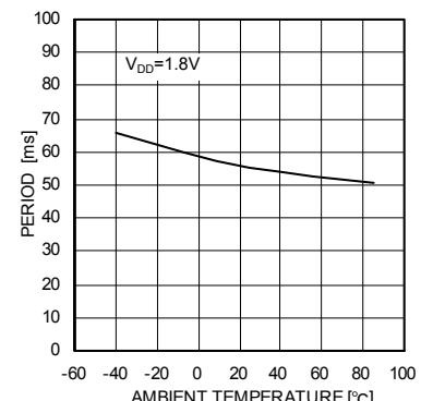
Fig.38 T<sub>P</sub> – Ambient temperature
