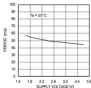
Fig.9 T<sub>P</sub>– Supply voltage
