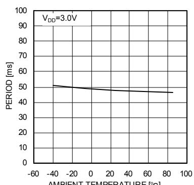
Fig.50 T<sub>P</sub> – Ambient temperature
