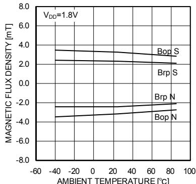
Fig.18 Bop,Brp – Ambient temperature
