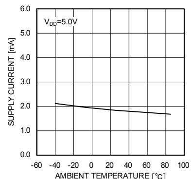
Fig.56 I<sub>DD</sub> – Ambient temperature
