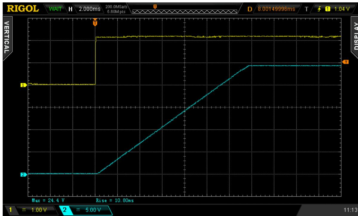
Figure 4. Typical Turn ON operation waveform for  $V_{IN} = 24\text{ V}$ ,  $C_{SLEW} = 18\text{ nF}$ ,  $C_{LOAD} = 10\mu\text{F}$ ,  $R_{LOAD} = 100\Omega$
