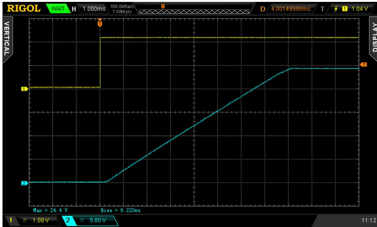
Figure 3. Typical Turn ON operation waveform for  $V_{IN} = 24\text{ V}$ ,  $C_{SLEW} = 10\text{ nF}$ ,  $C_{LOAD} = 10\mu\text{F}$ ,  $R_{LOAD} = 100\Omega$
