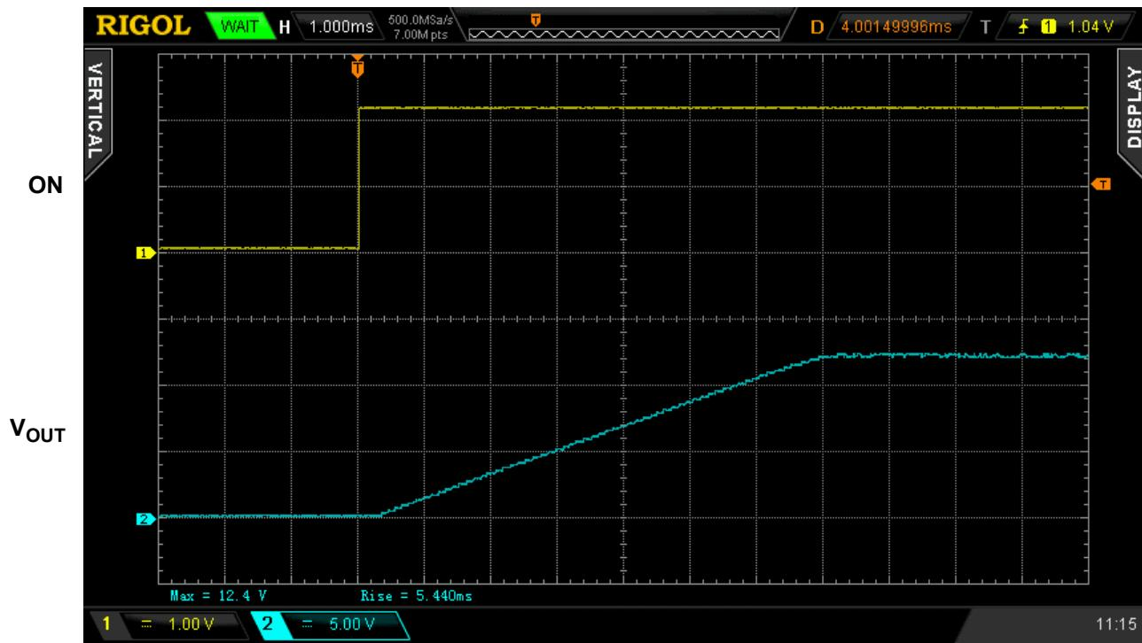
Figure 2. Typical Turn ON operation waveform for  $V_{IN} = 12\text{ V}$ ,  $C_{SLEW} = 18\text{ nF}$ ,  $C_{LOAD} = 10\text{ }\mu\text{F}$ ,  $R_{LOAD} = 100\text{ }\Omega$
