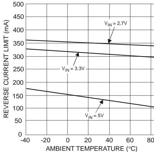
Fig. 6 Reverse Current Limit vs.
