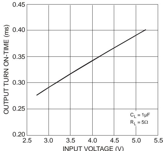
Fig. 3 Output Turn On-Time vs. Input Voltage
