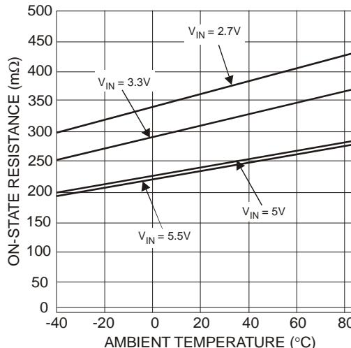
Fig. 4 Switch On-Resistance vs.
