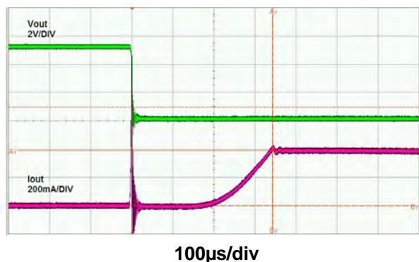
Deglitch Time from Reverse-Current Trigger to MOSFET Turn-Off
