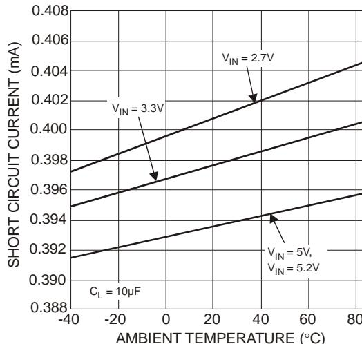
Fig. 2 Short Circuit Current Limit vs.
