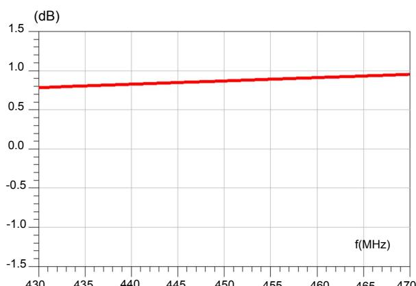
**Figure 4. Phase imbalance**
