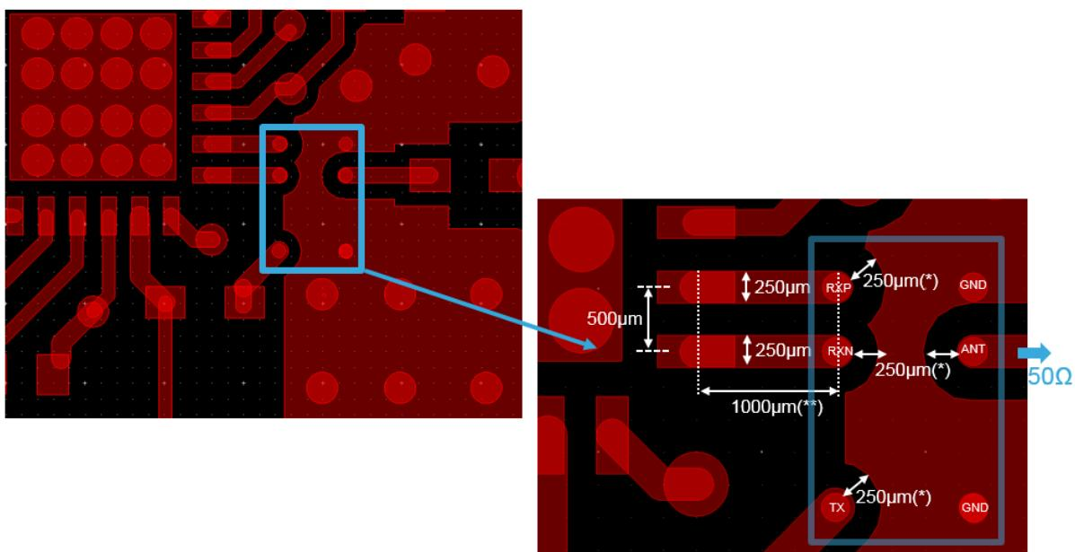
Note: (\*)Clearance 250 µm is needed to ensure good sensitivity.
