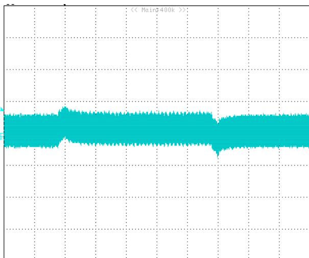
**Figure 18:** Typical transient response, 11.0Vin/1.8Vo
