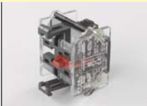
Contact block, screw terminal, slow-make (positive-break) with silver forced opening contacts
