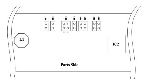
The following table shows the function of No 1 and No 2 of JP4, JP2, JP9. CU40025-UW6J is no reset inputs and M68 CPU bus parallel interface at default setting. Reset input signal is active when it is low.
