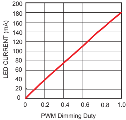
LED Current vs. PWM Dimming Duty
