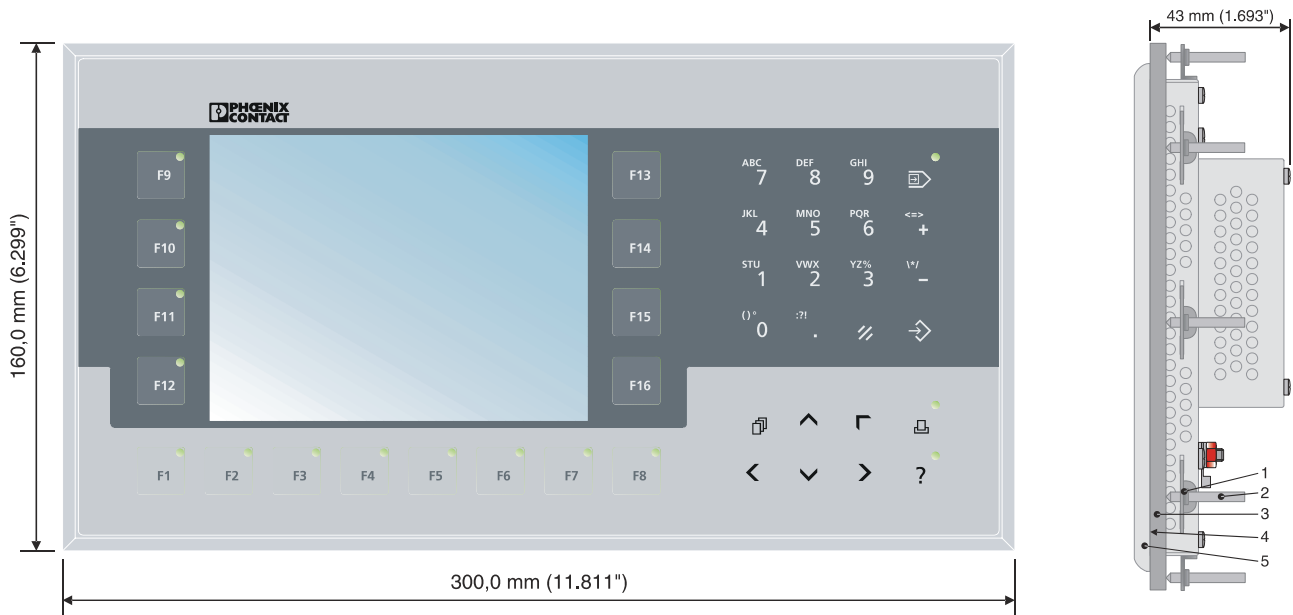
Figure 4 Front and side view of the OT 6M with dimensions
