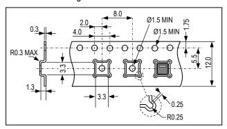
**Figure 22** Sketch of packaging tape and sensor orientation. Header tape is to the right and trailer tape to the left on this sketch.
