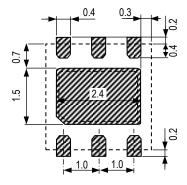
**Figure 8** Recommended metal land pattern for SHT2x. Values in mm. Die pad (centre pad) may be left floating or be connected to ground, NC pads shall be left floating. The outer dotted line represents the outer dimension of the DFN package.
