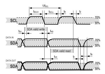
**Figure 12** Timing Diagram for Digital Input/Output Pads, abbreviations are explained in Table 5. SDA directions are seen from the sensor. Bold SDA line is controlled by the sensor, plain SDA line is controlled by the micro-controller. Note that SDA valid read time is triggered by falling edge of anterior toggle.
