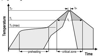
**Figure 9** Soldering profile according to JEDEC standard.  $T_P \le 260^{\circ}\text{C}$  and  $t_P \le 30\text{sec}$  for Pb-free assembly.  $T_L \le 220^{\circ}\text{C}$  and  $t_L \le 150\text{sec}$ . Ramp-up/down speeds shall be  $\le 5^{\circ}\text{C/sec}$ .
