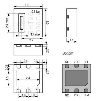
**Figure 1:** Drawing of SHT20 sensor package, dimensions are given in mm (1mm = 0.039inch), tolerances are  $\pm 0.1$ mm. The die pad (center pad) is internally connected to VSS. The NC pads must be left floating. VSS = GND, SDA = DATA. Numbering of E/O pads starts at lower right corner (indicated by notch in die pad) and goes clockwise (compare Table 2).
