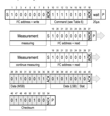
**Figure 16** No Hold master communication sequence – grey blocks are controlled by SHT2x. If measurement is not completed upon "read" command, sensor does not provide ACK on bit 27 (more of these iterations are possible). If bit 45 is changed to NACK followed by Stop condition (P) checksum transmission is omitted.
