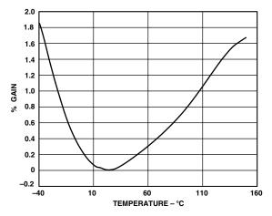
Figure 8. Gain Variation (from 25°C) vs. Temperature (–2000 ppm Field; R1 = 12  $k\Omega$ )
