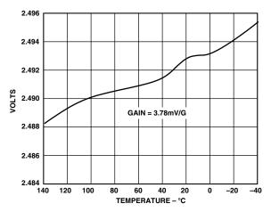
Figure 16. Absolute Offset Volts vs. Temperature
