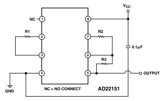
Figure 1. Typical Bipolar Configuration with Low (< -500 ppm) Compensation
