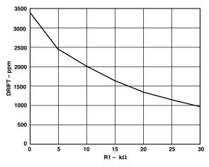
Figure 10. Drift Compensation (Pins 1 and 3) vs. Typical Resistor Value R1
