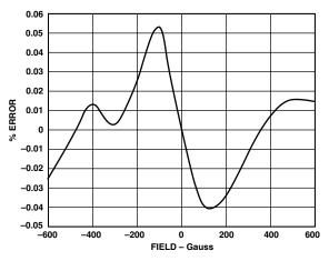
Figure 15. Integral Nonlinearity vs. Field
