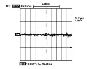
Figure 14b. Peak-to-Peak 180 Hz Bandwidth (10 mV/Division)
