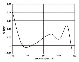
Figure 6. Gain Variation from 25°C vs. Temperature (–200 ppm) Field; R1 –15  $k\Omega$
