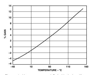
Figure 4. Uncompensated Gain Variation (from 25°C) vs. Temperature
