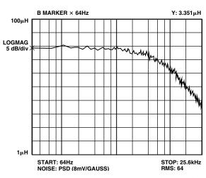
Figure 12. Power Spectral Density (5 mV/G)
