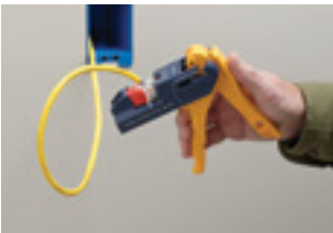
4. Ensure jack is completely and securely inserted in jack holder bed with IDC slots facing the blades.
