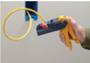
5. Pull trigger completely and remove excess wire prior to releasing trigger.
