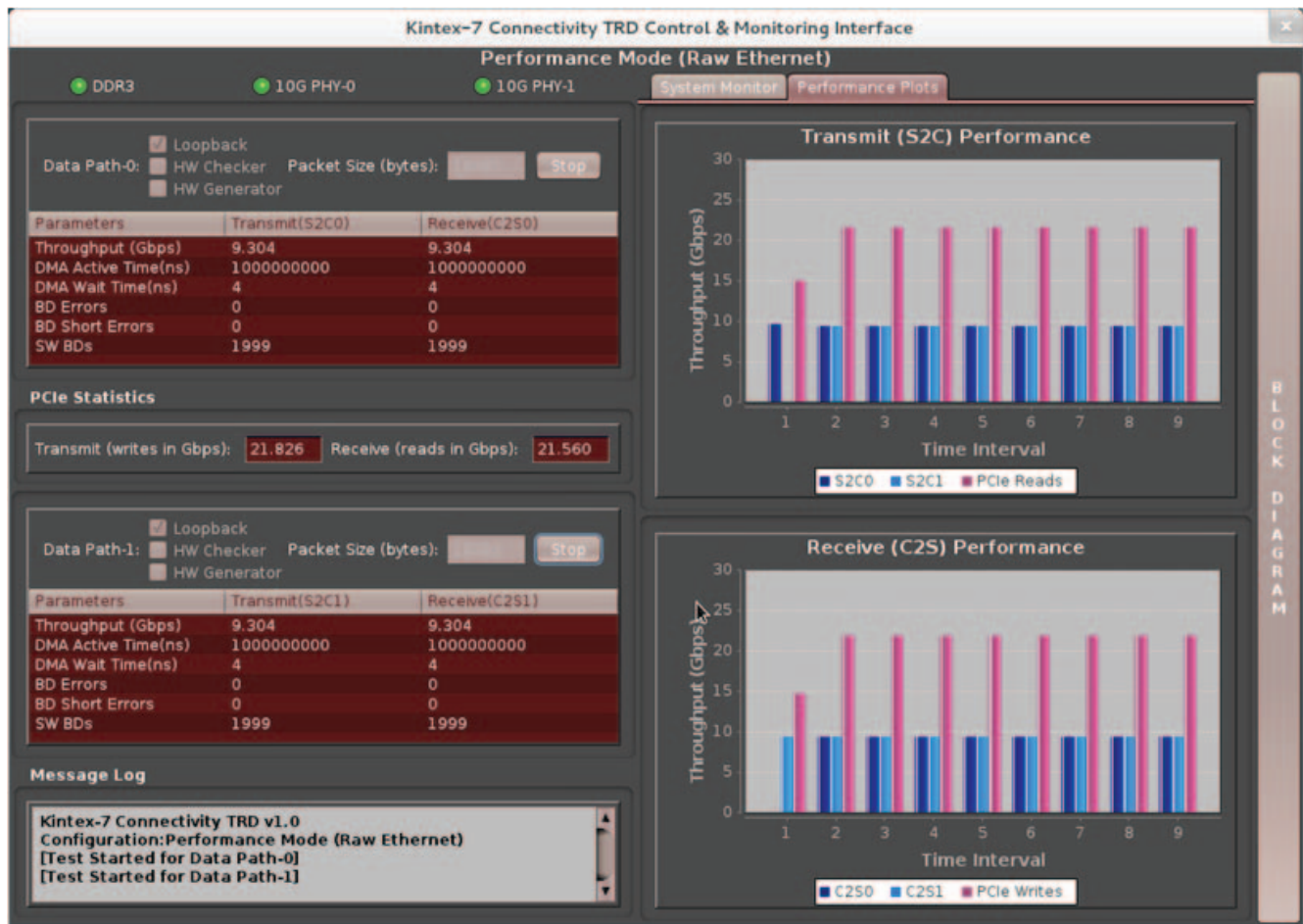
Figure 2-24: Raw Ethernet Driver Performance Plots
