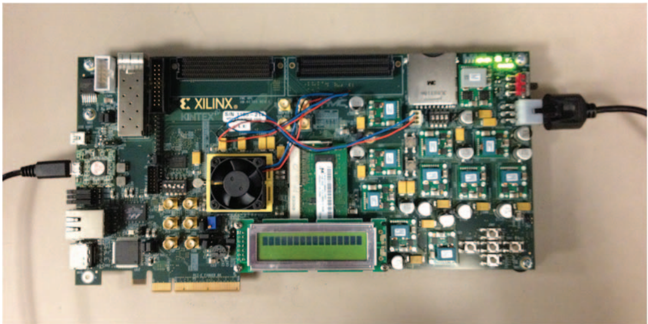
Figure 2-29: Cable Installation for KC705 Board Programming
