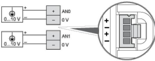
The (-) poles are connected internally.
