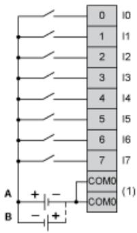
(1) The COM0 terminals are connected internally.
