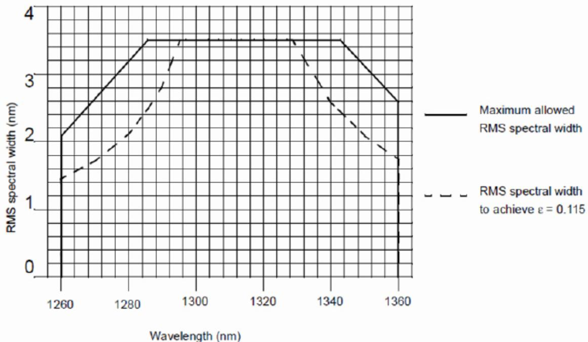
**Figure 59-3—1000BASE-LX10 Transmitter spectral limits**
