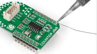
Turn the board upward again. Make sure to align the headers so that they are perpendicular to the board, then solder the pins carefully.
