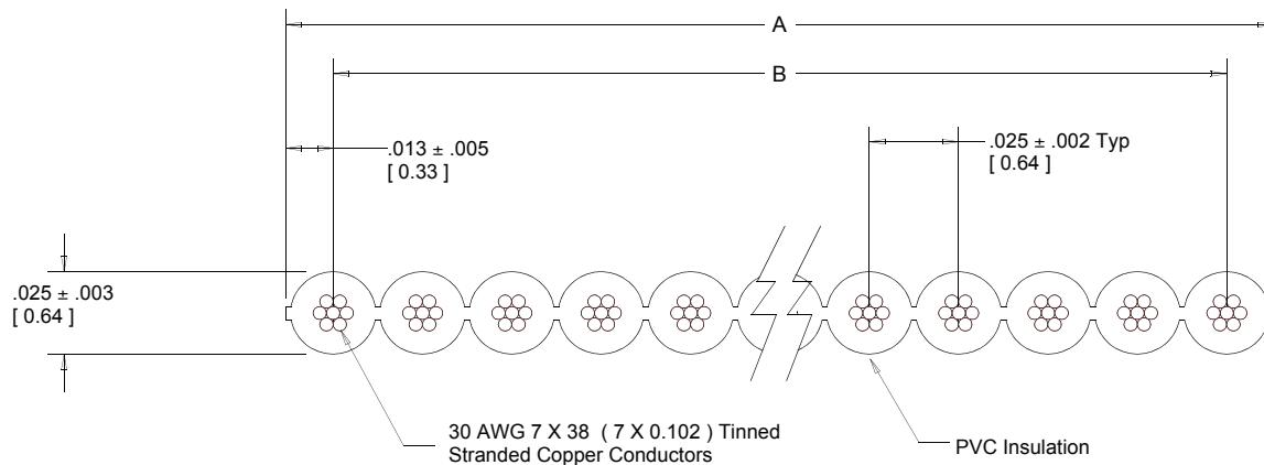
Note: Red marking on one edge of cable designates wire #1.
