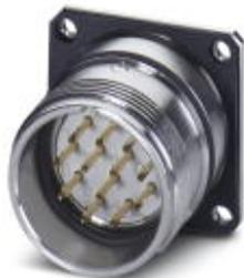
Device connector for rear wall, straight, Screw locking, M23, No. of pos.: 6, type of contact: Pin, Solder-in connection, Flat gasket, 4xM3, Panel thickness min.: 2.7 mm, Panel thickness max.: 3.5 mm
