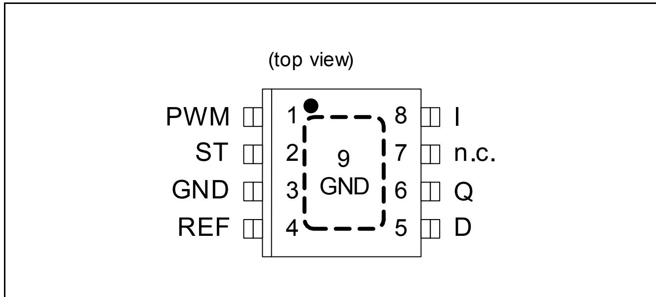
Figure 3-1 Pin Configuration
