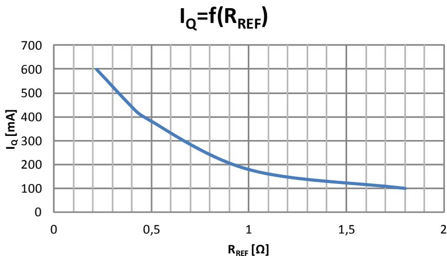
Figure 5-3 Output Current  $I_Q$  versus Reference Resistor  $R_{REF}$  with  $V_Q = 6.6$  V
