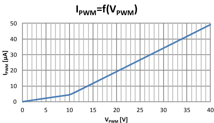
Figure 5-6 PWM Pin Input Current  $I_{PWM}$  versus PWM Voltage  $V_{PWM}$  at  $T_j = 25^\circ\text{C}$  and  $V_i = 13.5 \text{ V}$
