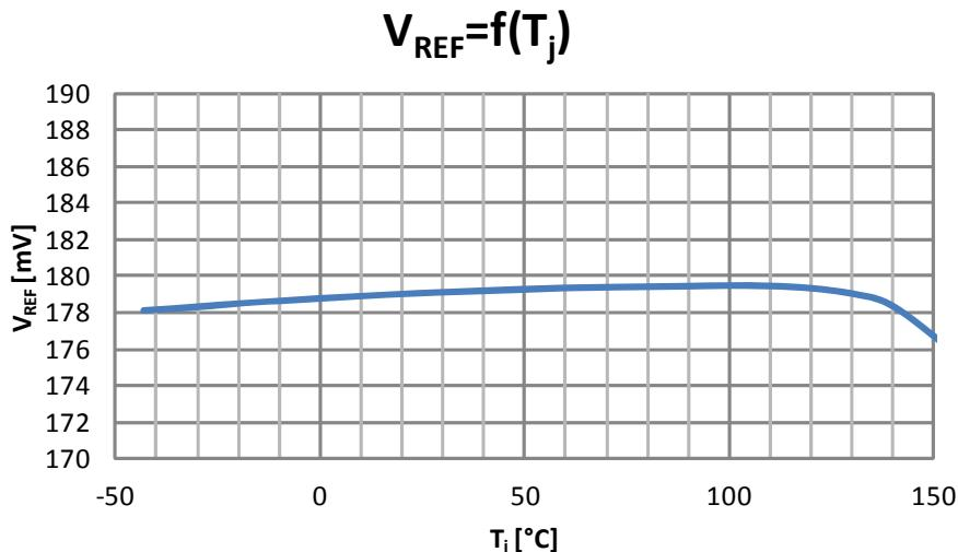
Figure 5-5 Reference Voltage  $V_{REF}$  versus Junction Temperature  $T_j$
