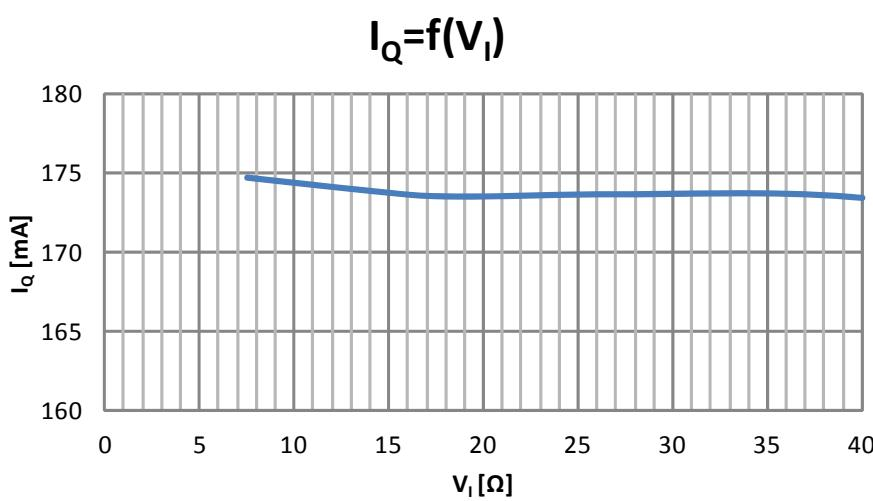
Figure 5-4 Output Current  $I_Q$  versus Supply Voltage  $V_I$  with  $V_Q - VREF = 6.6$  V and  $R_{REF} = 1$   $\Omega$
