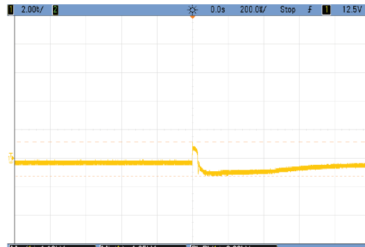
Output voltage waveform (Differential mode 0.90KV)
