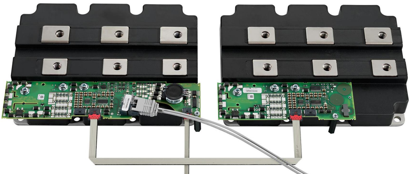
Fig. 1 1SP0635V (master, left) with 1SP0635D (slave, right) each screwed onto a 3.3kV IGBT module
