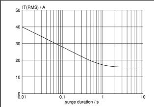
Fig.5. Maximum permissible repetitive rms on-state current  $I_{T(RMS)}$ , versus surge duration, for sinusoidal currents, f = 50 Hz;  $T_{hs} \le 38 \, ^{\circ}\text{C}$ .
