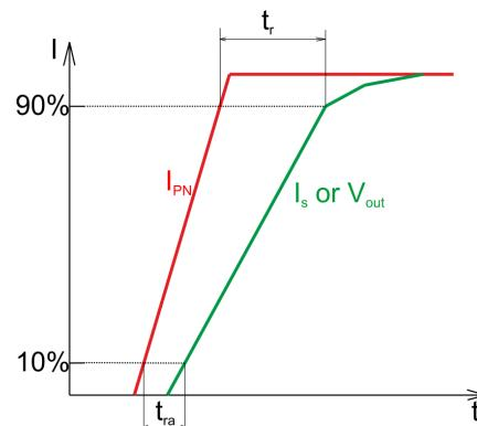
$t_r$ : Response time, measured as a delay time between a rectangular primary current and the output current  $I_S$  at  $I_P = 0.9 * I_{\text{PN}}$
