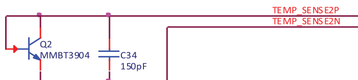
Figure 8.5. NPN Temperature Sensor Circuit
