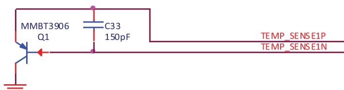
Figure 8.4. PNP Temperature Sensor Circuit
