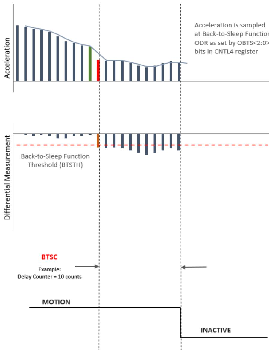
**Figure 14:** Latched Motion Interrupt Response with BTSC
