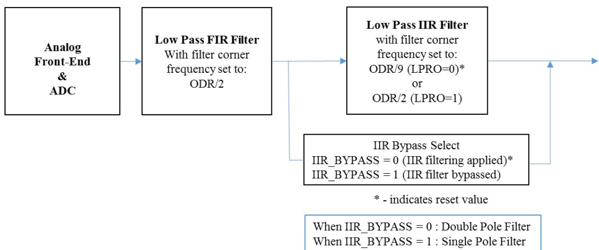
**Figure 10: Low-Pass Filter Design and Control Circuitry**
