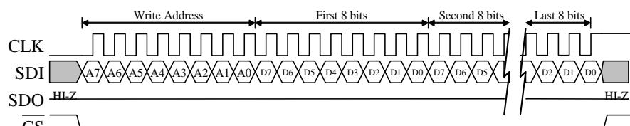
**Figure 5:** Timing Diagram for 8-Bit Register Write Operation
