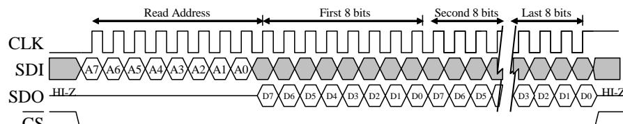
**Figure 6:** Timing Diagram for 8-Bit Register Read Operation
