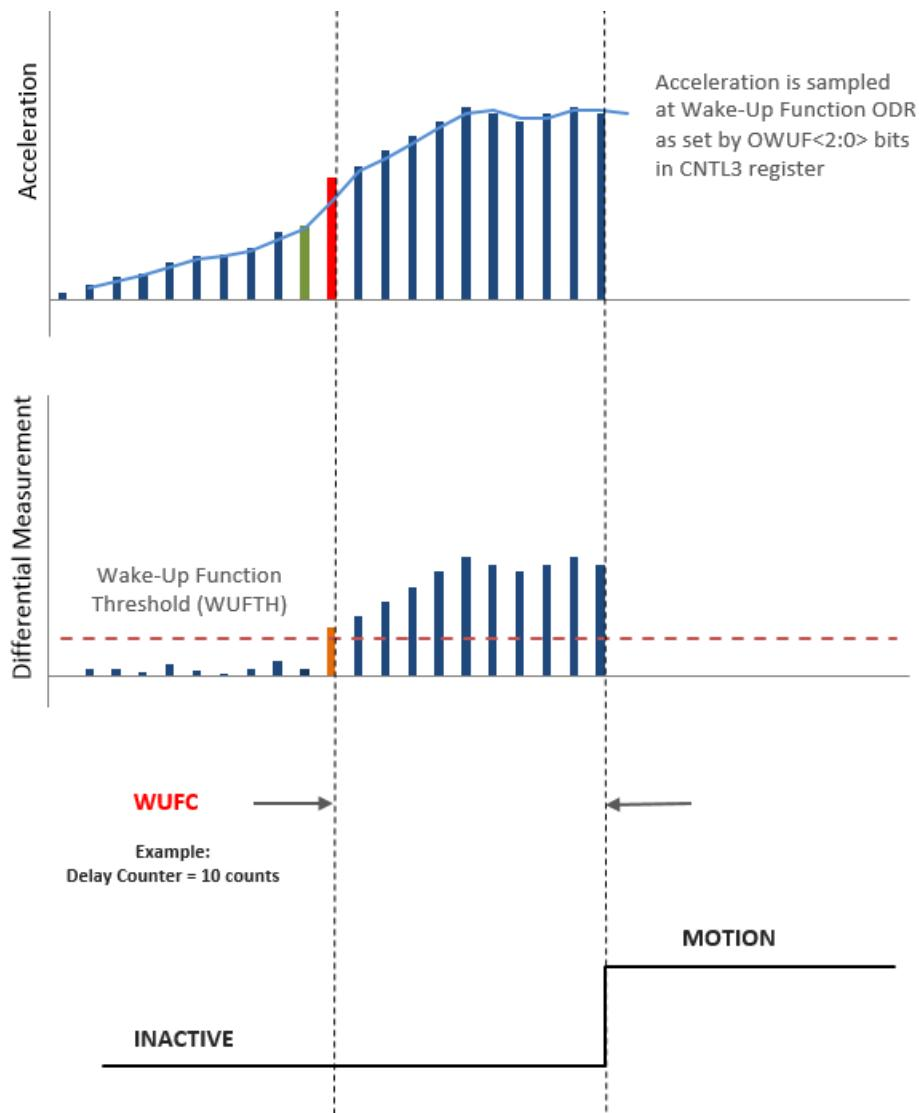
**Figure 13:** Latched Motion Interrupt Response with WUFC
