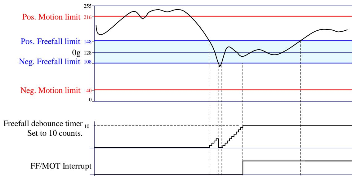
**Figure 19:** Typical Free fall Interrupt Example (FFCNTL ULMODE = 0)
