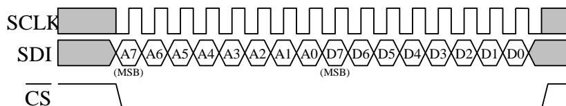
Figure 8: Timing Diagram for 8-Bit Register Write Operation
