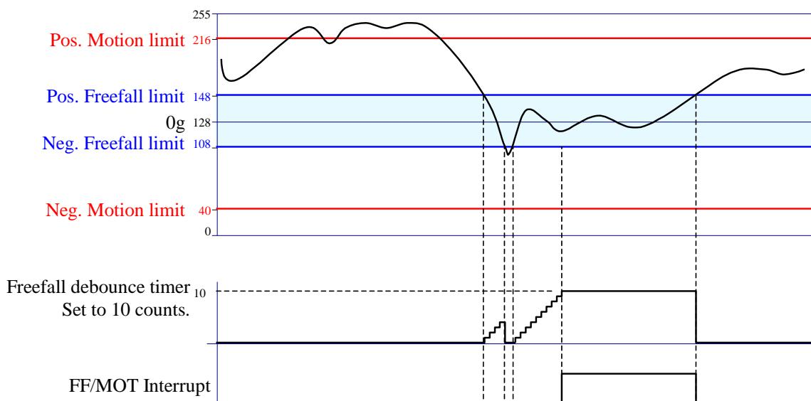
**Figure 18:** Typical Free fall Interrupt Example (FFCNTL ULMODE = 1)
