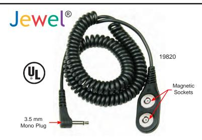
Jewel® MagSnap Coil Cords meet or exceed the requirements of ANSI/ESD S20.20 and ANSI/ESD S1.1 including section 5.4 Breakaway Force "With the ground cord connected to the cuff in a normal manner, a force of  $\geq$  .45 kg (1 lb) but  $\leq$  2.3 kg (5 lb) applied to the ground cord, in the normal disconnect direction, shall be required to separate the ground cord from the cuff."
