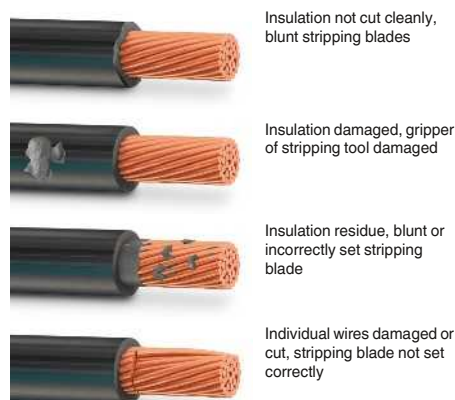
Cable stripped incorrectly according to DIN IEC 60352
