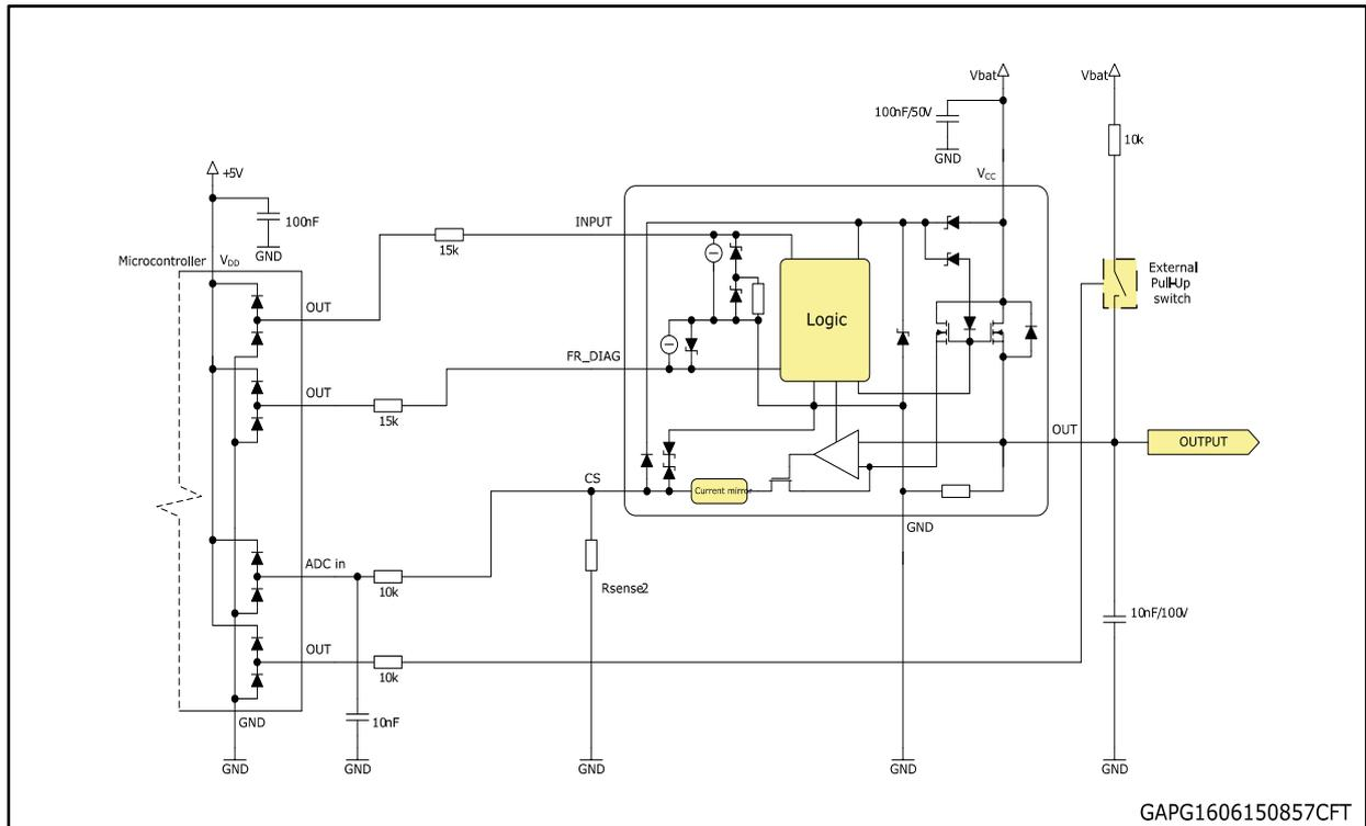
Figure 33: Open-load / short to VCC condition
