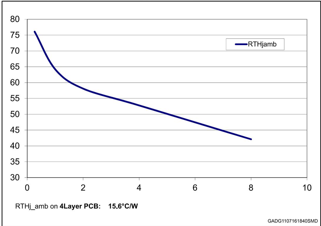
Figure 38: Octapak thermal impedance junction ambient single pulse
