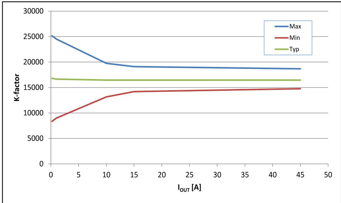
Figure 5: Current sense precision vs. I<sub>OUT</sub>
