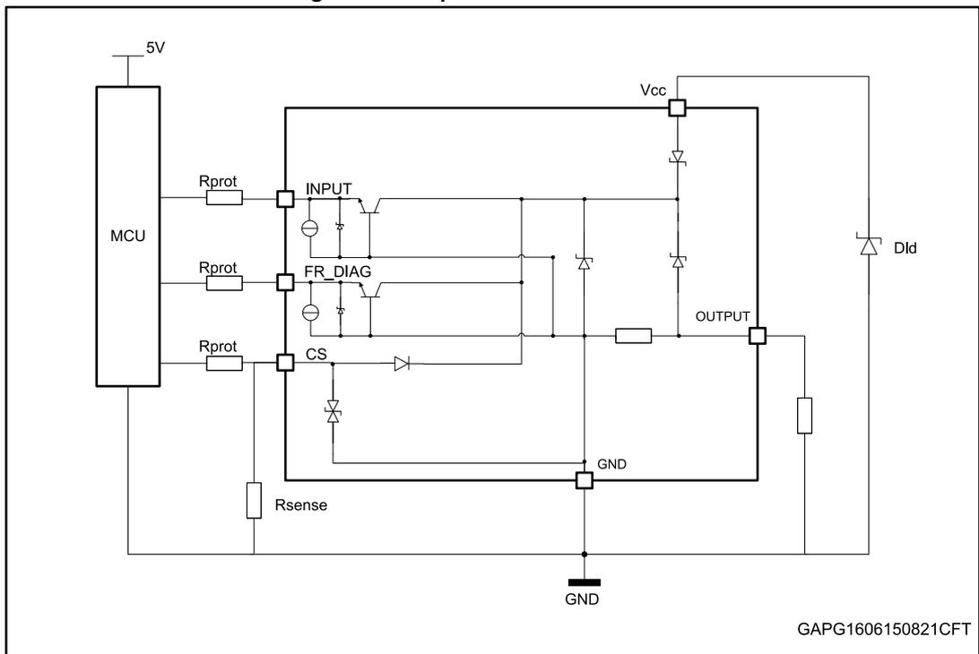
The device does not need any external components to protect the internal logic in case of a reverse battery condition. The protection is provided by internal structures.
