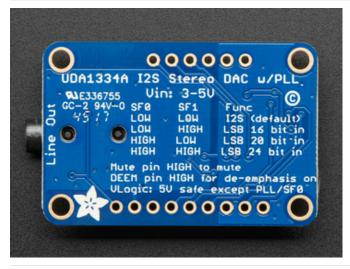
**SFO** and **SF1** are used to set the input data format. By default both are pulled Low for I2S but you can change them around for alternate formats.
