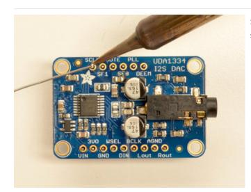
Solder each one of the pins into the board to make a secure connection
