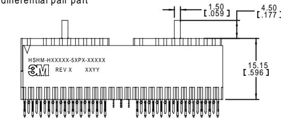
Coaxial, column differential and stripline configuration shown with protective caps\*
