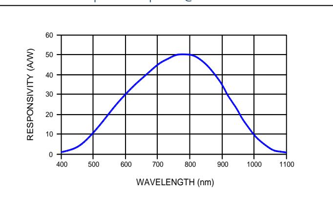
**ELECTRO-OPTICAL CHARACTERISTICS @ 23° C (V<sub>CC</sub> = single supply +3.3V, R<sub>L</sub> = 100W unless otherwise specified)**
