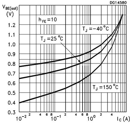
Figure 8. Base-Emitter Saturation Voltage (PNP)
