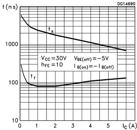
Figure 14. Resistive Load Switching Time (PNP)
