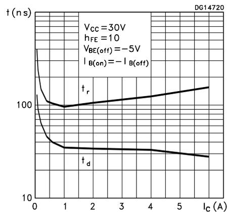
Figure 13. Resistive Load Switching Time (NPN)
