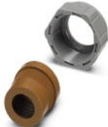
Half screw connection Pg21, made of plastic, consisting of rubber seal with one hole and one pressure screw, for type 2 - 4 housings, cable [mm] 14 - 18
